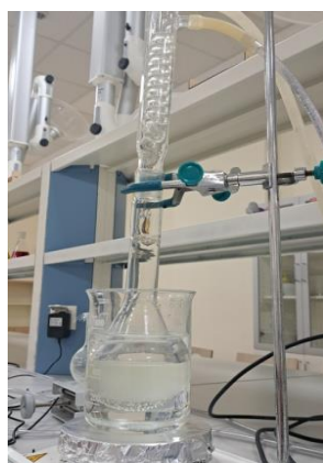
Figure 2. Esterification of fatty acids with ethanol
